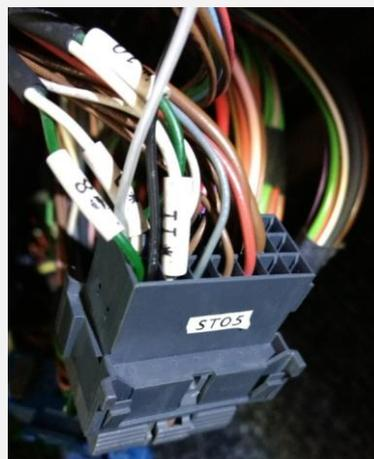
Figura 4 - Conector CAN ST05
