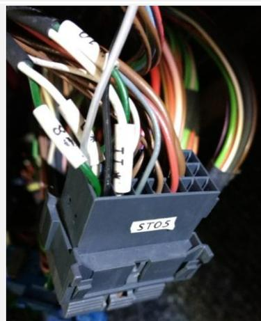
Figura 5 - Conector CAN ST05
